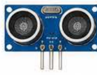
HC-SR04 Ultrasonic Sensor
