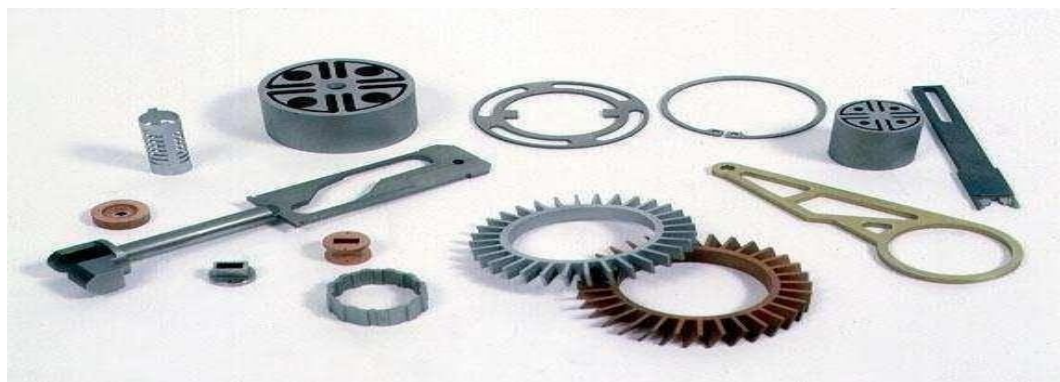
Figure: Difficult internal parts made by EDM process
