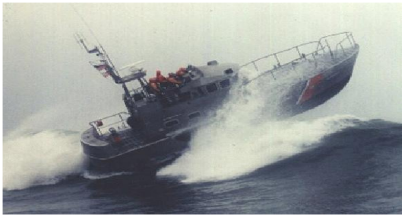
Fig.22 Pitching action of ship
