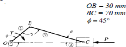
Figure 5.5(A) Graphical force analysis of a slider crank mechanism, which is acted on by piston force P and crank torque T
