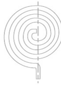
(b) Spiral torsion spring.
