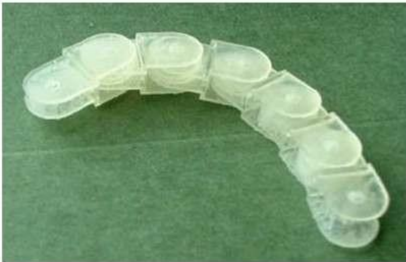
Pulley-driven snake-like robot Source: Gibson.
