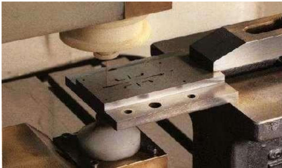
Figure 4: Wire erosion of an extrusion die
