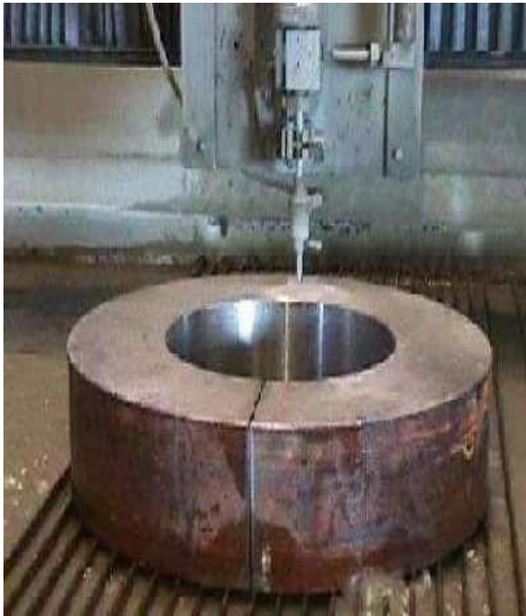
Abrasive water jet cutting
