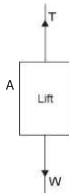
Fig. 8.7. Lift moving upwards.
