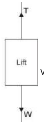
Fig. 8.8. Lift moving downwards.
