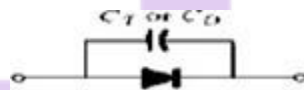
Fig 1.17: Including the effect of the transition or diffusion capacitance on the semiconductor diode
