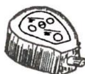
(h) 15 A, 3-Pin Switch Socket Combined
