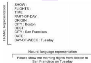
Fig. Q.19.1 : A sample user query and its frame representation in the ATIS program
