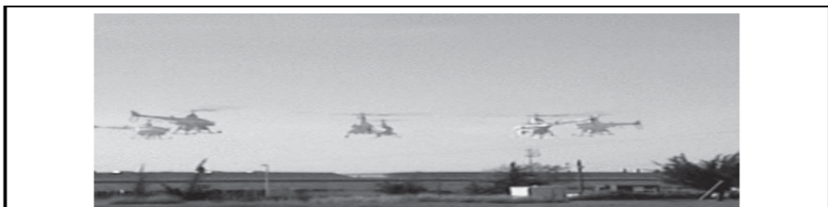
Figure 21.10 Superimposed time-lapse images of an autonomous helicopter performing a very difficult “nose-in circle” maneuver. The helicopter is under the control of a policy developed by the PEGASUS policy-search algorithm. A simulator model was developed by observing the effects of various control manipulations on the real helicopter; then the algorithm was run on the simulator model overnight. A variety of controllers were developed for different maneuvers. In all cases, performance far exceeded that of an expert human pilot using remote control. (Image courtesy of Andrew Ng.)
