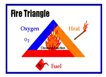
• of fuel and oxygen. If the concentration of a specific gas is below the lower explosive limit (LEL) it is too lean to burn. If the concentration is above the upper explosive limit (UEL) it is too rich to burn.
