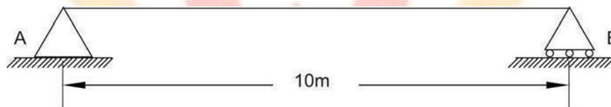
Figure 37.2: The beam structure
