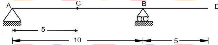
Figure 37.19: Overhang beam structure
