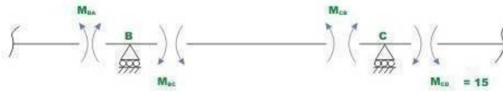
Fig. 14.6 b Free - body diagrams of joints B and C along with members
