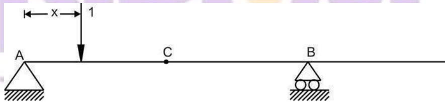
Figure 37.22: A unit load before section C
