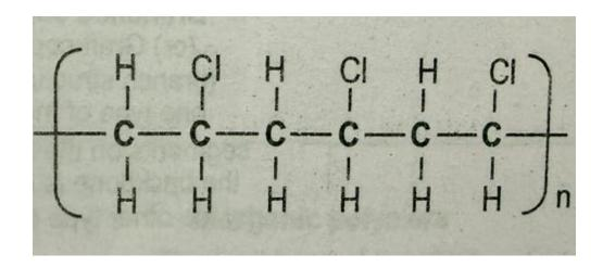
Atactic polymers: no regular arrangement of functional groups on the backbone of polymer chain.
