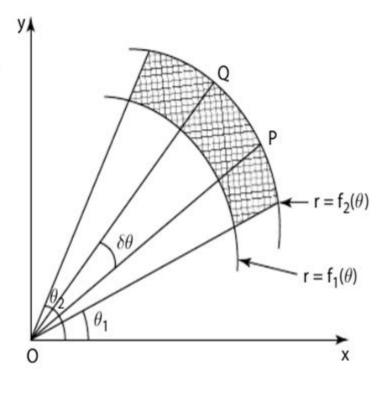
To evaluate  $\int_{\theta}^{\theta_2} \int_{r_1}^{r} f(r,\theta) dr d\theta$ , we first integrate w.r.to r between the limits  $r = r_1$  and  $r = r_2$  keeping  $\theta$  fixed and the resulting expression is integrated w.r.to  $\theta$  from  $\theta_1$  to  $\theta_2$
