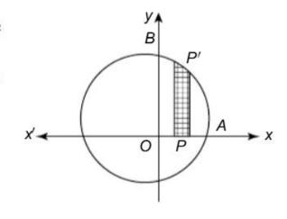
$$I = \int_{0}^{a} \int_{0}^{\sqrt{a^{2} - x^{2}}} xy dy dx = \int_{0}^{a} x \left(\frac{y^{2}}{2}\right)_{0}^{\sqrt{a^{2} - x^{2}}} dx = \frac{1}{2} \int_{0}^{a} (xa^{2} - x^{3}) dx$$
