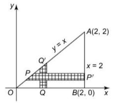
The region is covered by first moving along the horizontal strip PP' and then sliding this strip parallel to itself to from y = 0 and y = 2.
