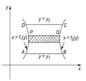
$$\int_{y_1}^{y_2} \int_{x_1}^{x_2} f(x, y) \, dx dy = \left[ \int_{y_1}^{y_2} \left[ \int_{x_1}^{x_2} f(x, y) \, dx \right] \, dy \right]$$
