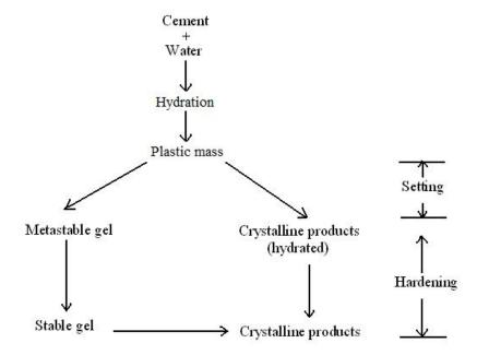
Chemical reactions involved in Setting and hardening of cement:
