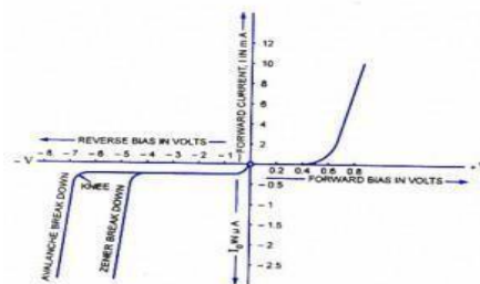
Figure 1.18: Diode characteristics with breakdown
