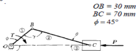
Figure 5.5(A) Graphical force analysis of a slider crank mechanism, which is acted on by piston force P and crank torque T
