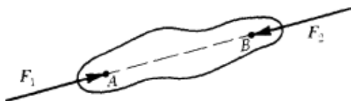
Figure 5.2(A) A two-force member. The resultant force and the resultant moment both equal Zero.
