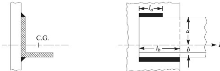
Fig. Axially loaded unsymmetrical welded section
