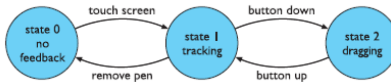
Figure 12.2 Light pen transitions: three states
